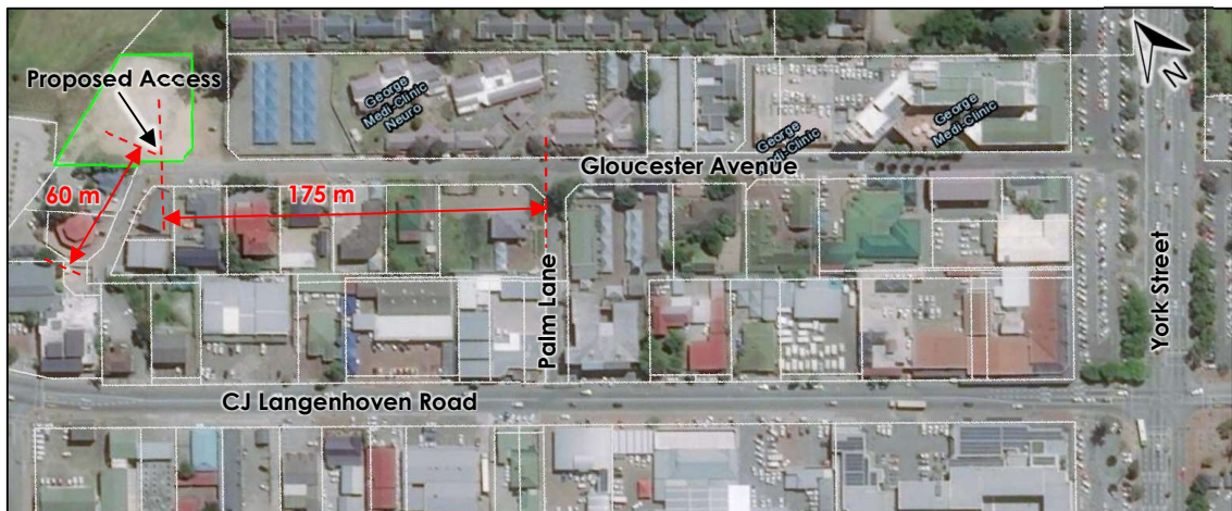
Figure 3.3 Available shoulder sight distance
