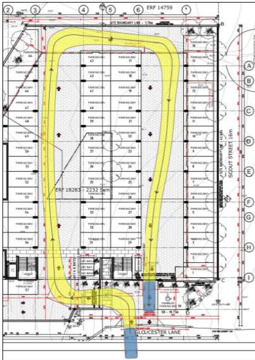
Figure 3.8 AutoTURN - Parking aisles (one-way section)
