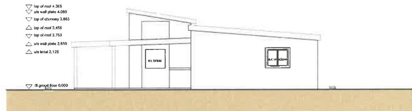
WEST ELEVATION - scale 1 : 100
