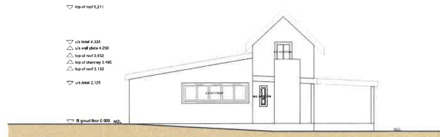
EAST ELEVATION - scale 1 : 100
