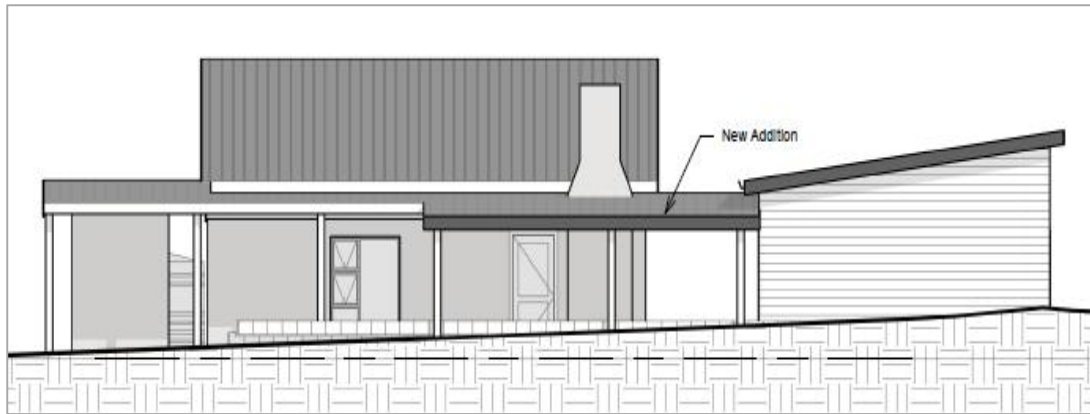
Figure 5 – New covered rear stoep
