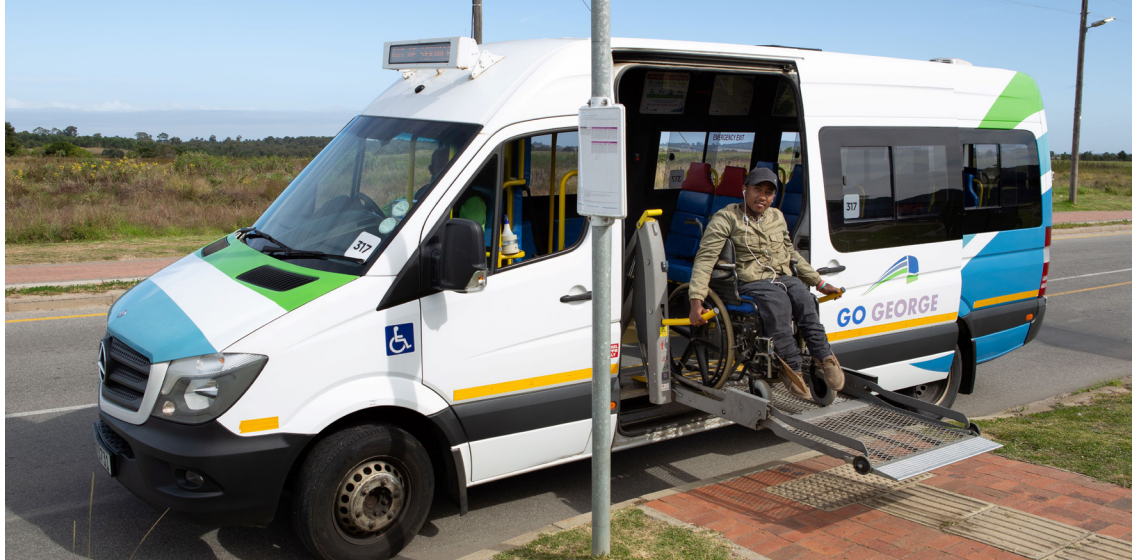
The minibus has been equipped with a hydraulic hoist giving access to passengers with mobility impairment.
