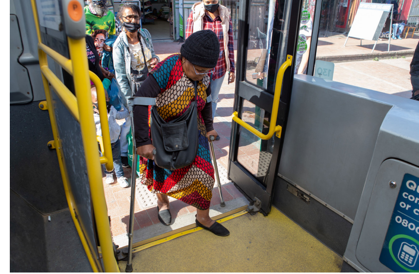
The larger buses can “kneel” to meet the elevated bus stop to accommodate passengers using mobility devices or who cannot comfortably step up to the bus entrance.
