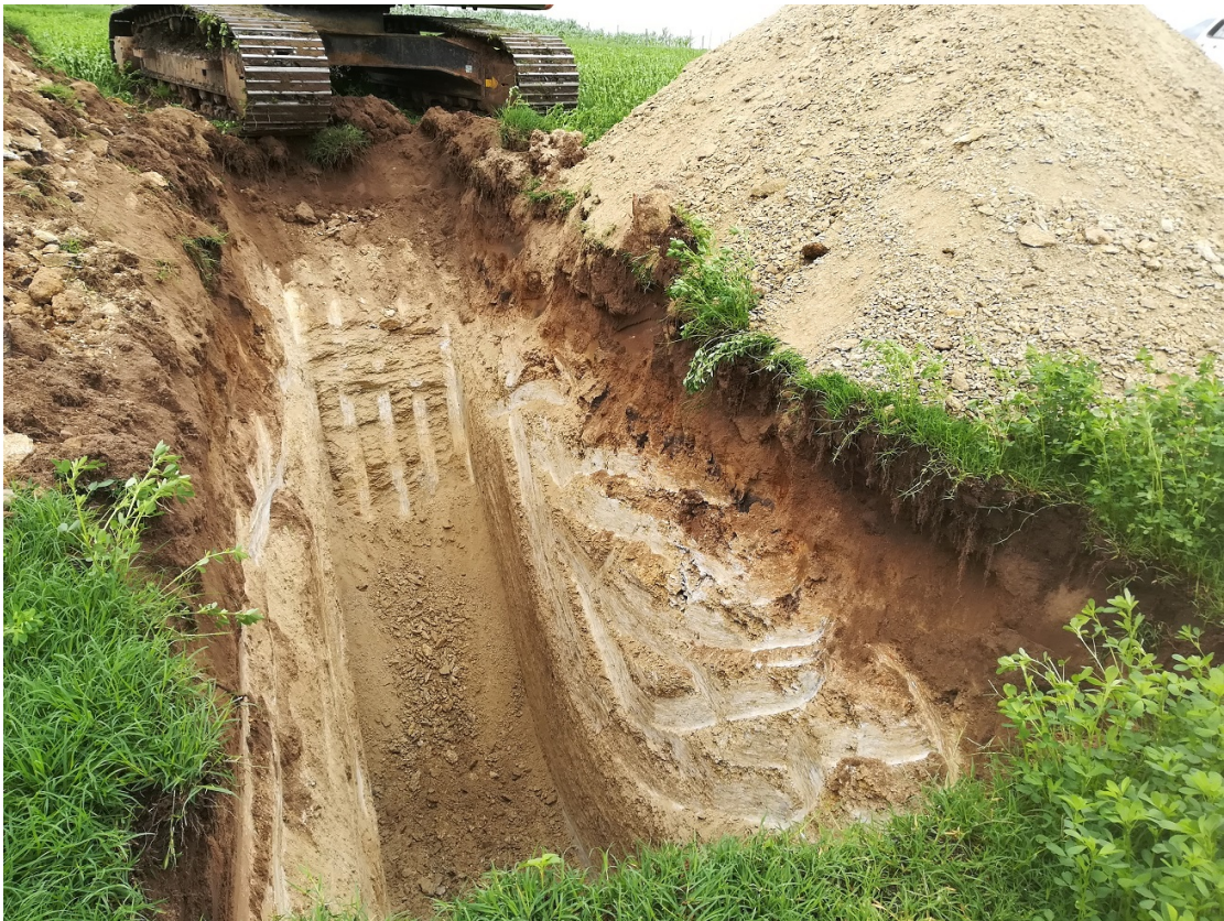
Figure 4. View of test pit showing soil and gravel conditions, plus gravel heap.
