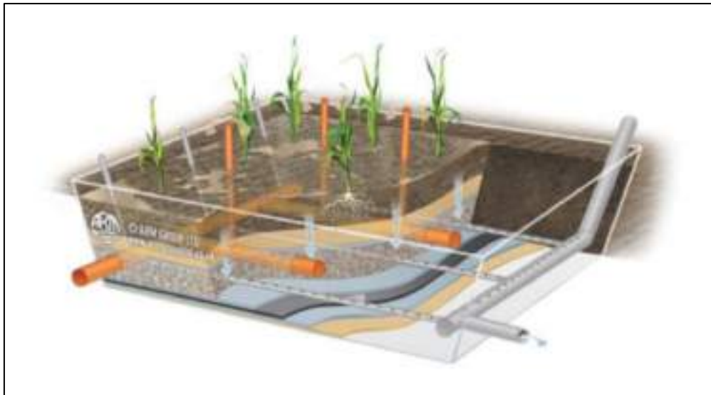
FIGURE 5: SLUDGE TREATMENT CONSTRUCTED WETLAND
