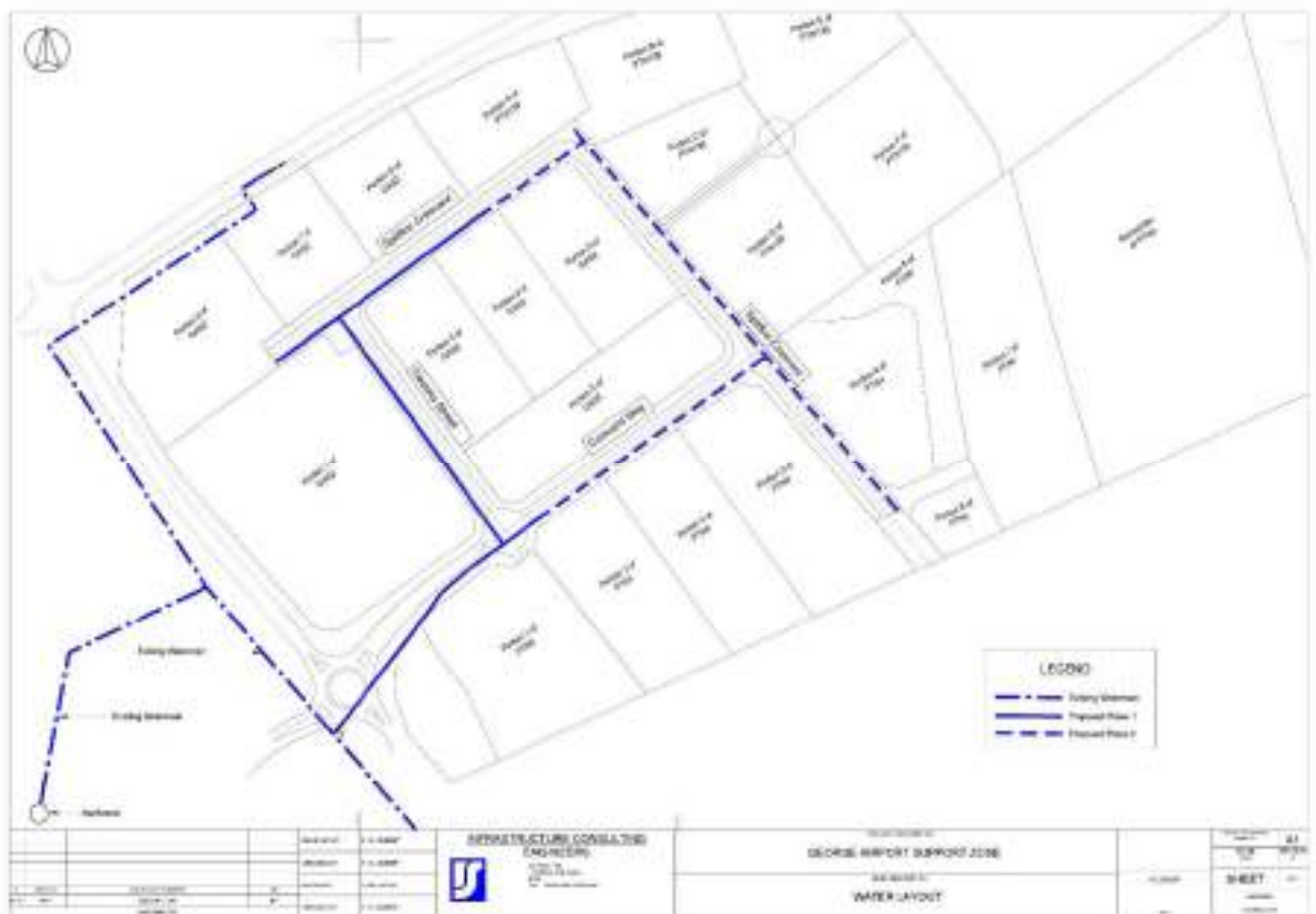
Figure 2: Services (water) required for Phase 1 of the development on Ptn 4, and for development on Ptns 130 to 132 (solid blue lines), connecting to the municipal bulk supply. The dotted blue lines are water lines needed for the next phase of development (ASZ plan).
