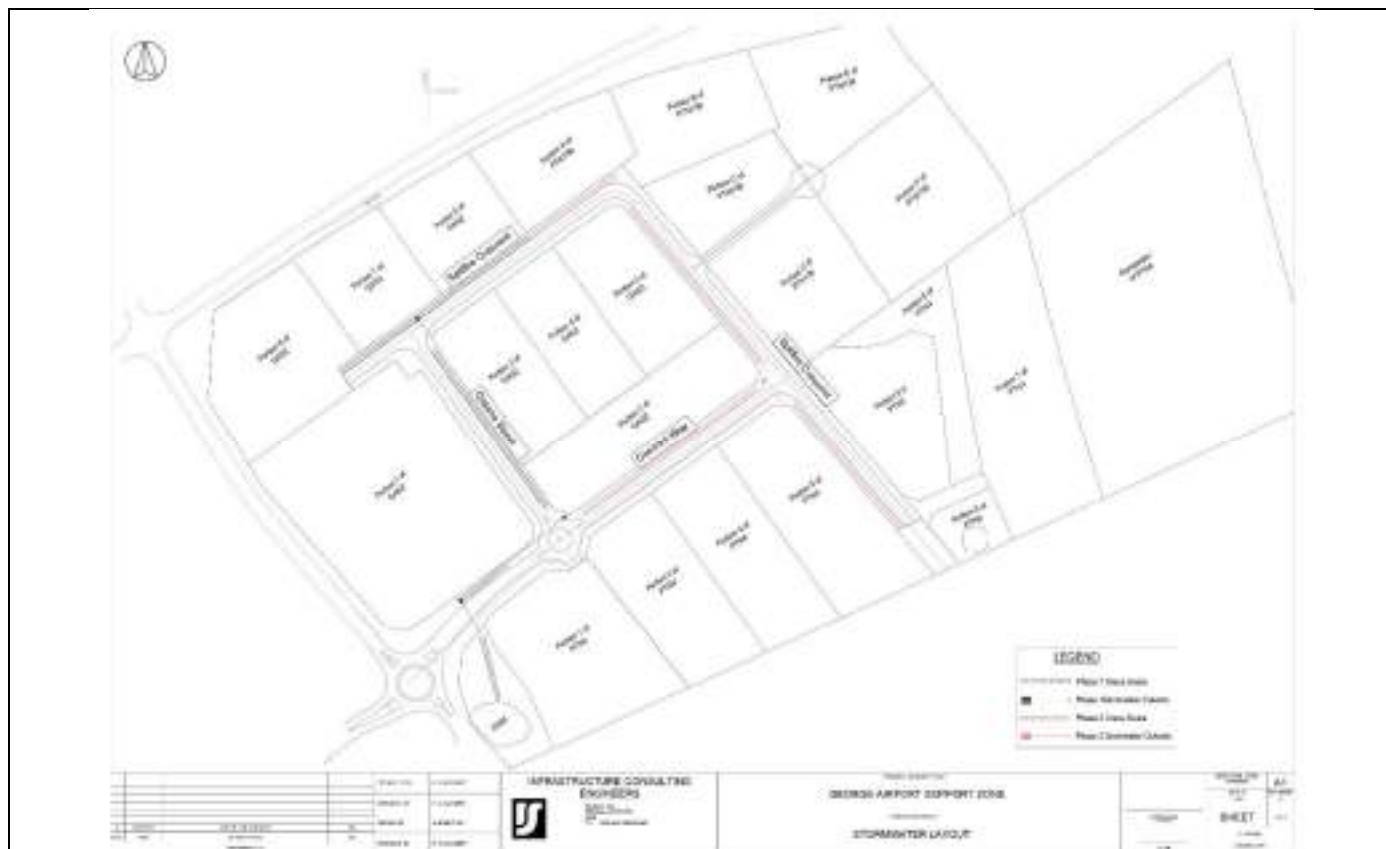
Figure 4: Stormwater infrastructure and grass swales required for Phase 1 of the development on Ptn 4, and for development on Ptns 130 to 132 (black lines. The red lines are stormwater infrastructure and grass swales needed for the next phase of development (ASZ plan).
