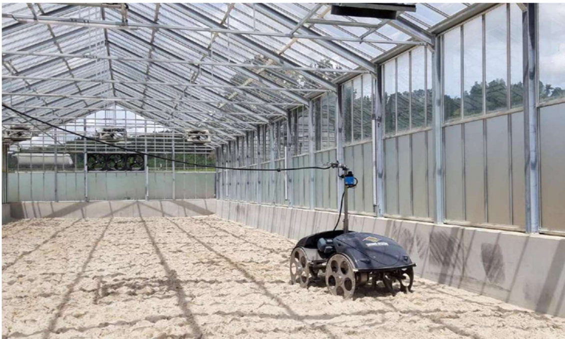
Figure 5: Electric mole as part Solar batch system (Thermo-Systems)
