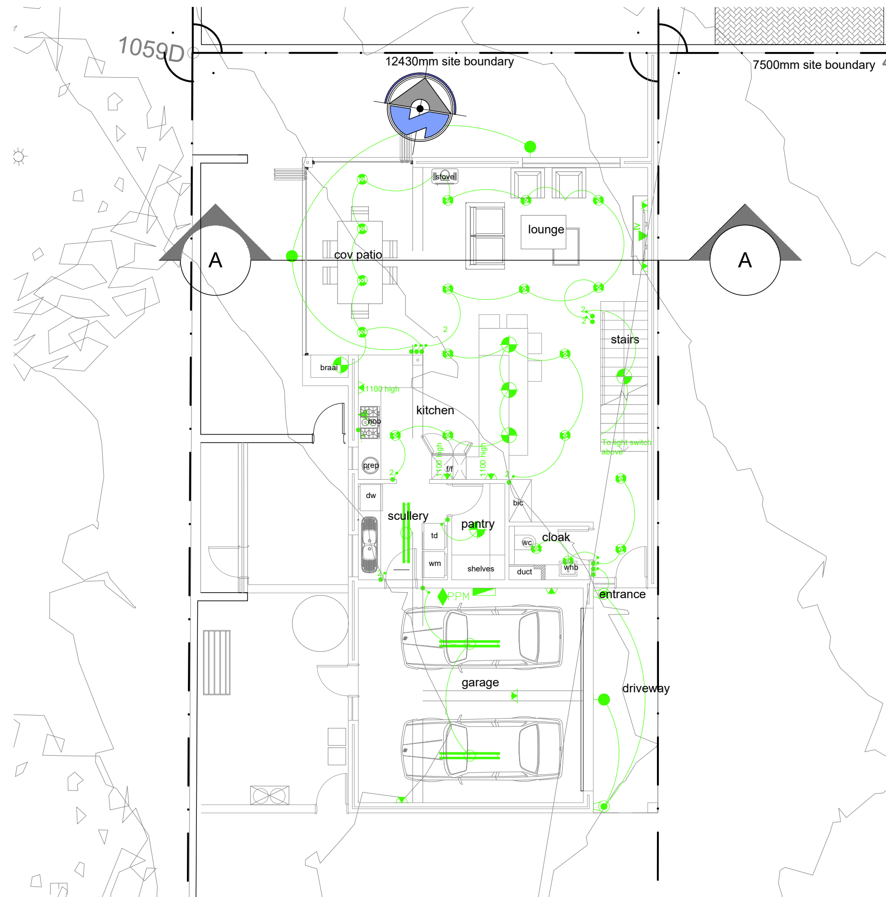
GROUND STOREY ELECTRICAL LAYOUT - scale 1 : 100
