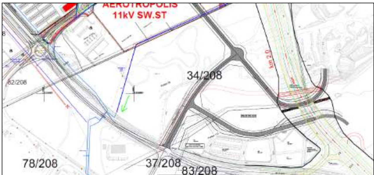
Figure 4: 11kV O/H line (proposed point of connection at green arrow)
