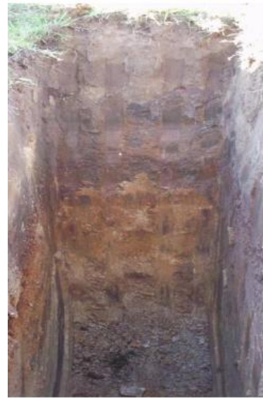
Silty sand and silty clay test pit no. 5
