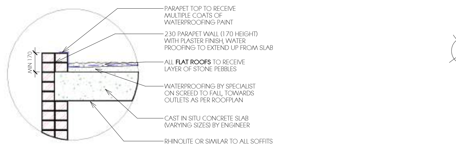
TYPICAL PARAPET WALL DETAIL 1:20
